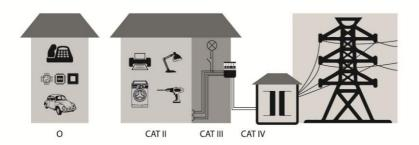
Overview of measurement categories according to IEC 61010-01 O = No Measurement Category (Other circuits that are not directly connected to mains)
